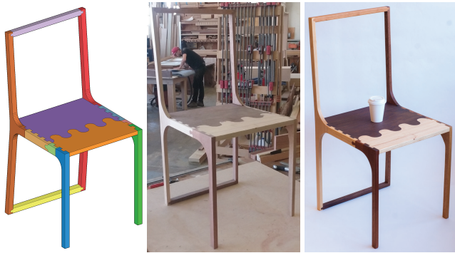
Fig. 14. We commissioned a woodworker to fabricate a version of the Branca chair at full size using the solid 3D parts generated by our tool. (Coffee cup added for scale.)
