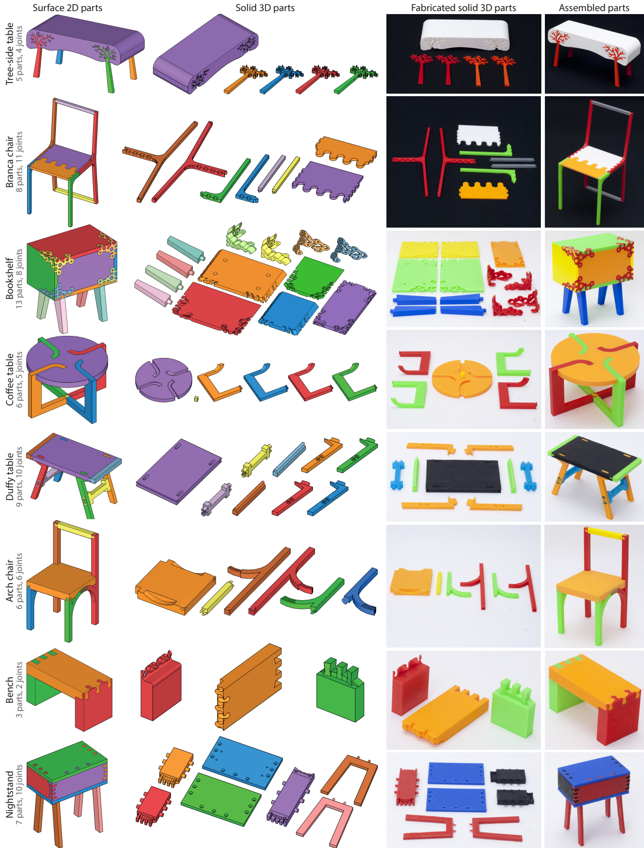
Fig. 12. Complete furniture assemblies we designed using our interactive tool. Please zoom in to see the geometry of the joints.
